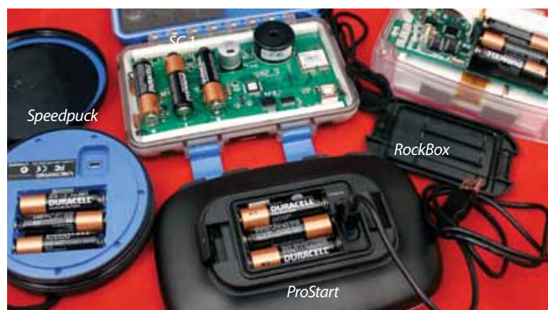
The Velocitek SpeedPuck and ProStart have sealed innards, but the Velocitek SC-1 and RockBox bare their circuit-board souls.
